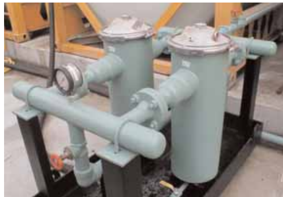
HEK11 filter sets continuously clean bulk oil at a copper mine in Indonesia. Read the case study details on the next page.
