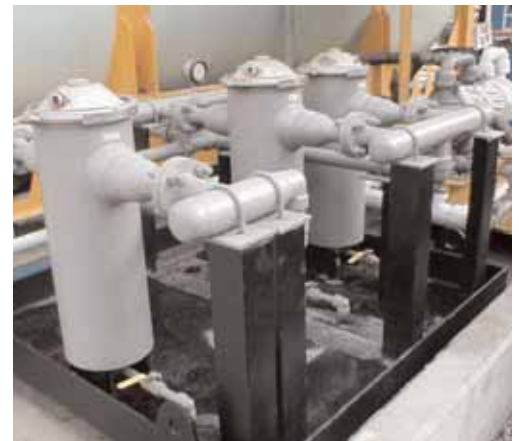
HEK11 filter sets continuously clean bulk oil at a copper mine in Indonesia. Read the case study details on the next page.
