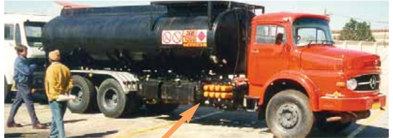
This truck transports hydraulic fluid to mines, steel mills and other industrial sites in South Africa. Four double-head HMK25 Duramax filters, with flow rates of 100gpm, are used to clean the oil before it is piped into large storage tanks at the customer site.
